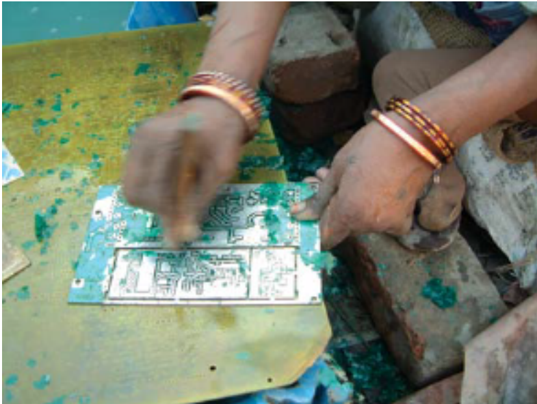
Recovering copper from printed circuit boards (Photo courtesy: EMPA)
